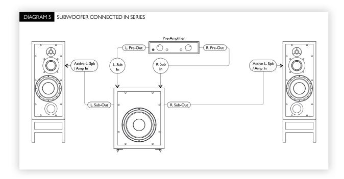
Diagram 5 – Typical Configuration – Stereo playback (Mono Sub). A preamplifier or AV receiver Output is connected to the L and R Inputs of the subwoofer. The subwoofer L and R Outputs are connected to the Input of the L and R main stereo amplifier or active loudspeakers. In this configuration the Gain switch is normally set to 0dB.
