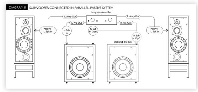
Diagram 7 and 8 – 2.1 Configuration – The subwoofer is driven by a preamplifier/AV receiver with a second pre-amplifier Output or dedicated subwoofer Output. Additional subwoofers may be daisy chained using the subwoofer Outputs, or connected in a stereo configuration as shown.
