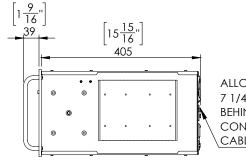
ALLOW 185MM / 7 1/4" CLEARANCE BEHIND FOR CONNECTOR & CABLE BEND RAD.
